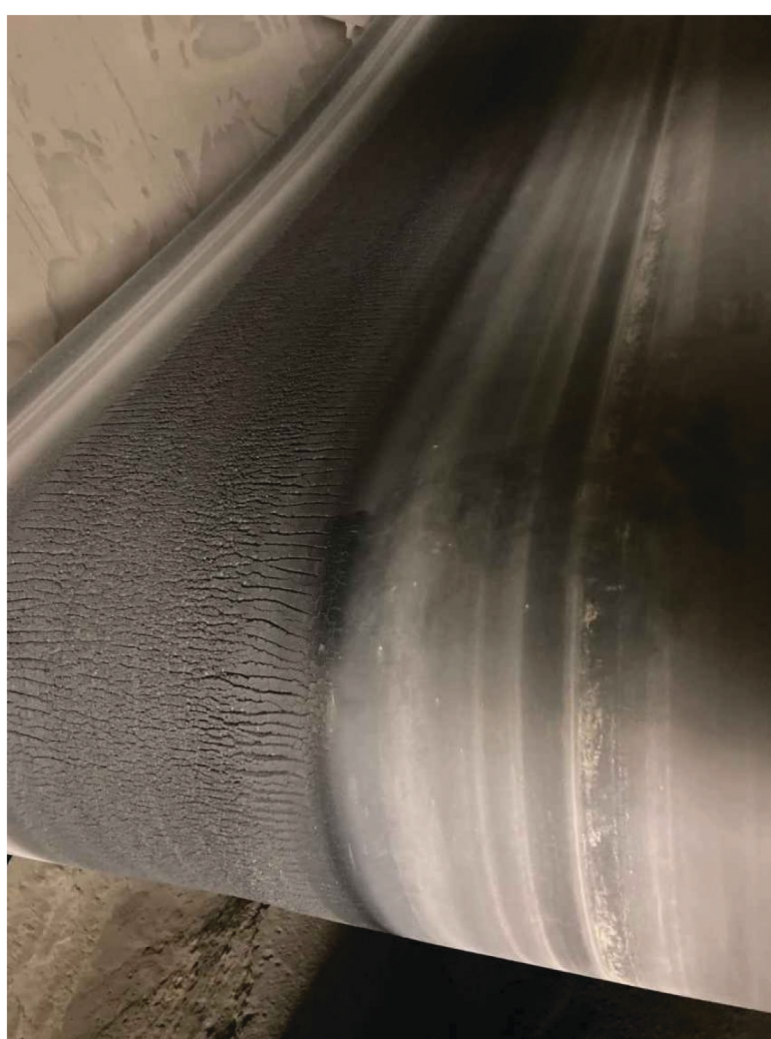
Omitting key ingredients to reduce costs causes life-limiting damage to the rubber
