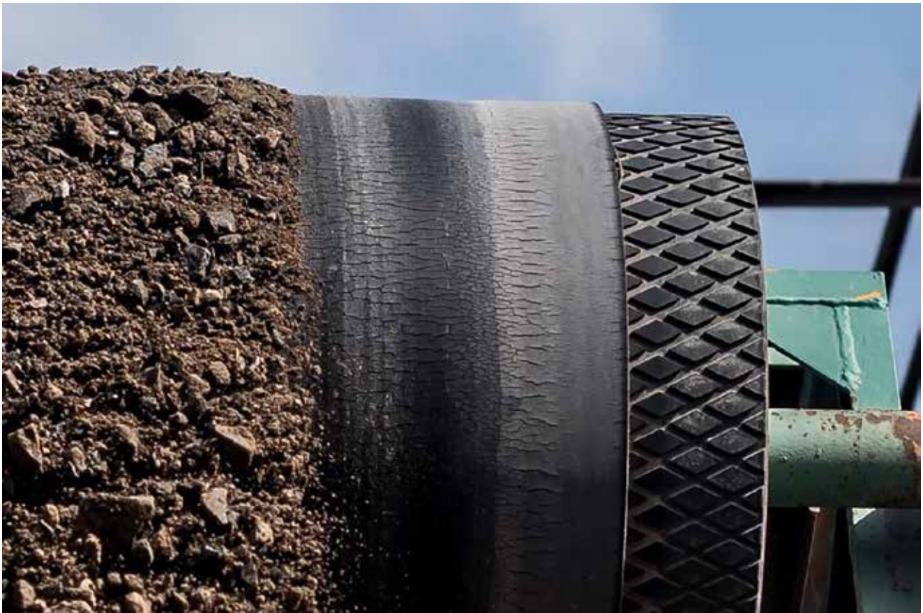
Belts that are not fully resistant to ozone and UV have a much shorter lifespan
