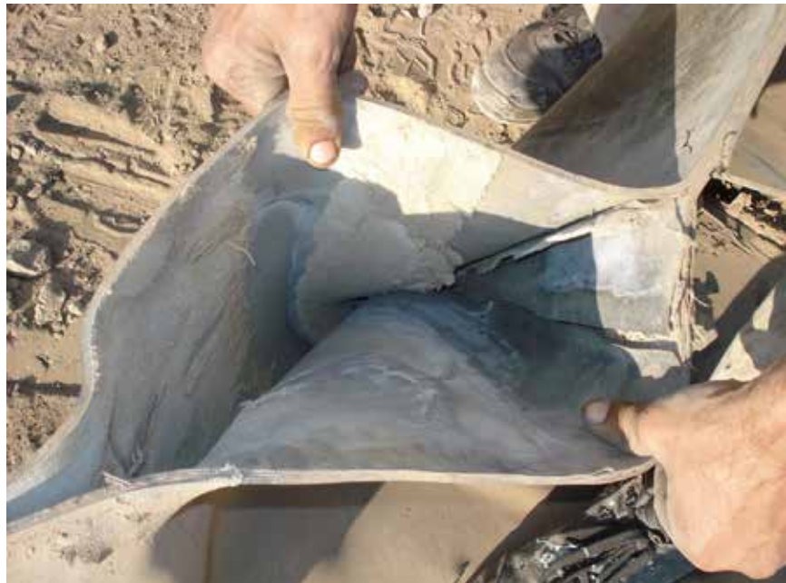
Delamination – layers separate and the belt literally falls apart.
