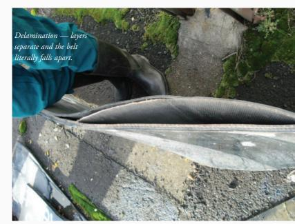
layers and between the surfaces of the outer plies and the rubber covers. Basically, it is what holds the conveyor belt together. Adhesion is defined as the force required to separate (pull apart) the adhesion between adjoining plies and/or between the plies and the outer covers. This is usually measured in Newtons per millimetre (N/mm).
