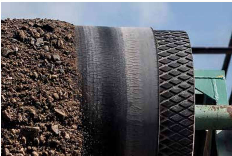
Pollution problems – fine particles of dust penetrate the cracks and are then discharged (shaken out) on the return (underside) run of the belt.
