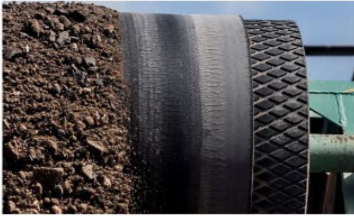
Figure 5. Surface cracking caused by ozone and ultraviolet.
